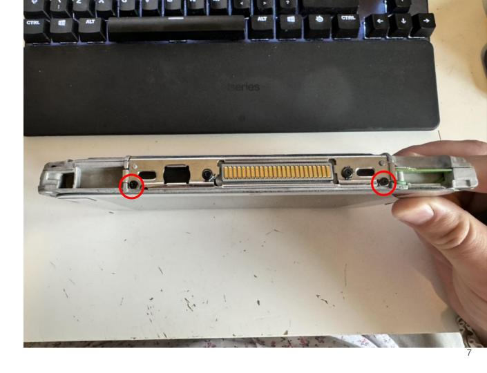
Remove the two screws holding on the battery latch
