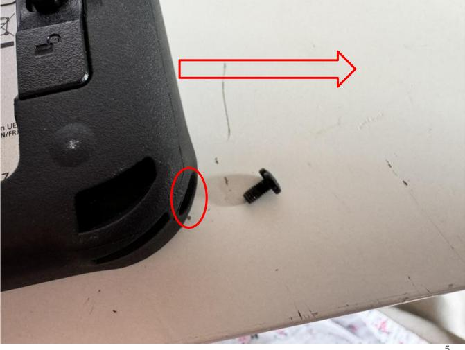
Remove the two screws next to the docking connector, then gently pry off the black plastic
