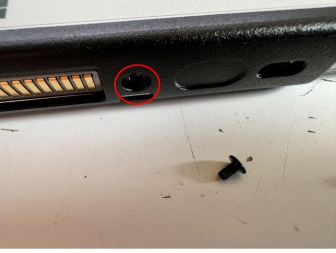
Remove the two screws holding on the metal around the docking connector
