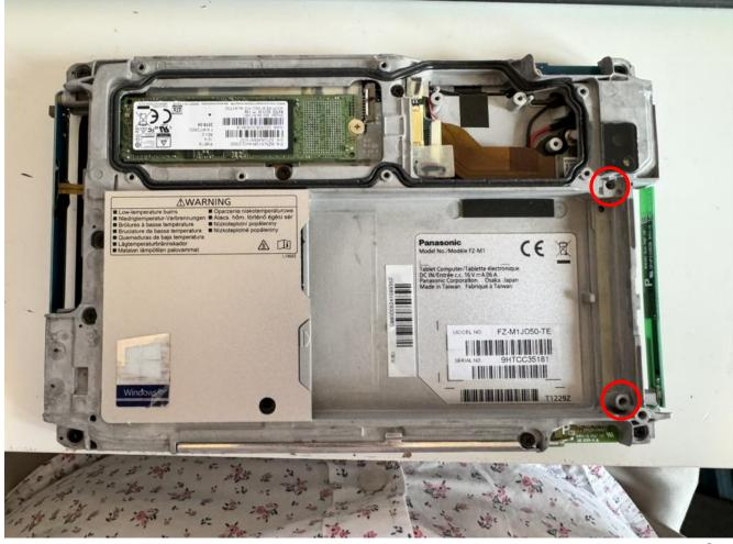
Remove the two screws on the button panel
