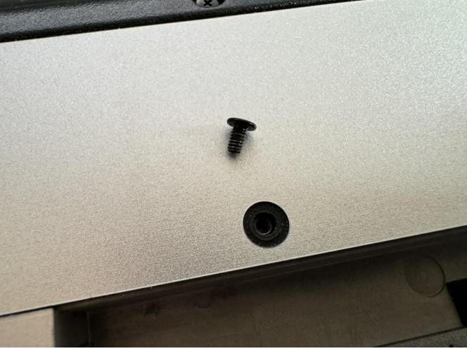
Here's the type of screw used in the bottom section (above the Micro SD Card / SIM Card slots)
